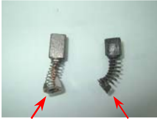
New Motor Brush Worn Motor Brush (Fig 26)
