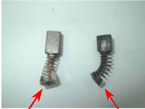
New Motor Brush Worn Motor Brush (Fig 26)
