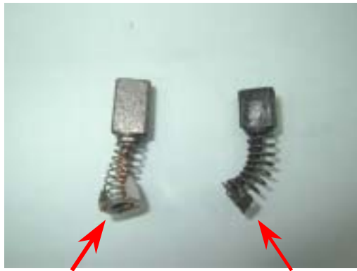
New Motor Brush Worn Motor Brush
