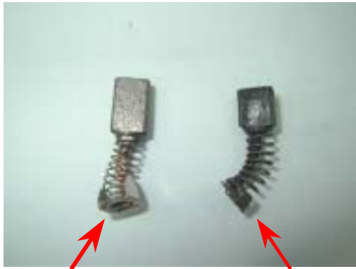
New Motor Brush Worn Motor Brush (Fig 19)
