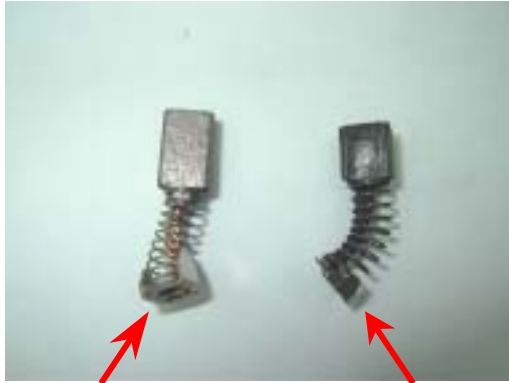
New Motor Brush Worn Motor Brush (Fig 18)
